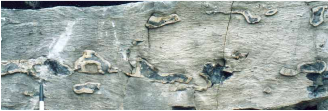
Photo 5. Location 2-b, wall beside apartments off Brittany Drive. 4cm pen top. Irregular shaped chert nodules in limestone block. White margins are calcareous whereas black cores are very finely crystalline quartz.
